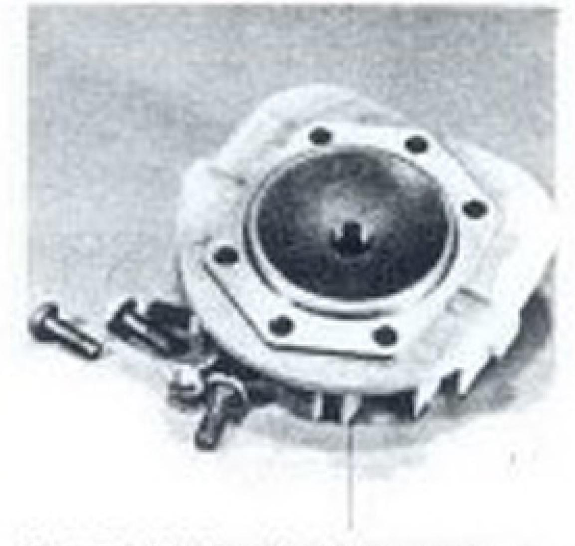
LEFT - Although there appears to be an eight screw head hold-down pattern, only six screws are actually used. This is discussed in the text.
